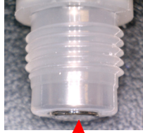
Glass sensing surface protruded relatively to the outer body (view without gas membrane)
