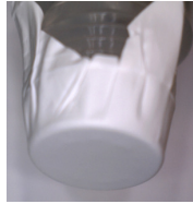
Membrane on outer body without the inner sensing stem (retaining cap not shown)
