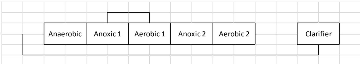
The University of Cape Town (UCT) process includes anaerobic, anoxic, aerobic, and anoxic reactors in series with aerobic mixed liquor recycle to the second stage anoxic reactor, first stage anoxic mixed liquor recycle to the anaerobic reactor, and return sludge recycle to the first stage anoxic reactor. Figure 5 illustrates the UCT process.
