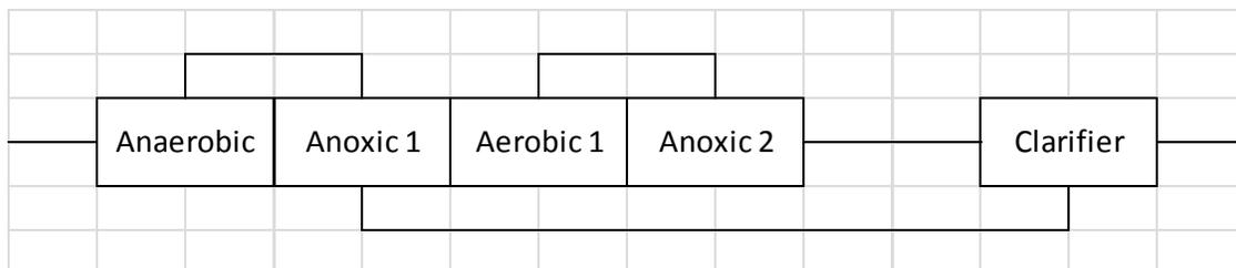
The Virginia Initiative Plant (VIP) process includes anaerobic, anoxic and aerobic reactors in series with aerobic mixed liquor recycle to the anoxic reactor, anoxic reactor mixed liquor recycle to the anaerobic reactor, and return sludge recycle to the anoxic reactor. Figure 6 illustrates the VIP process.
