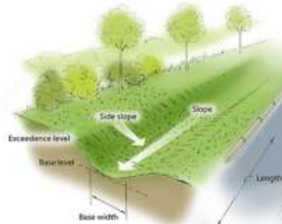
Vegetated Slope. Source: XP Drainage
